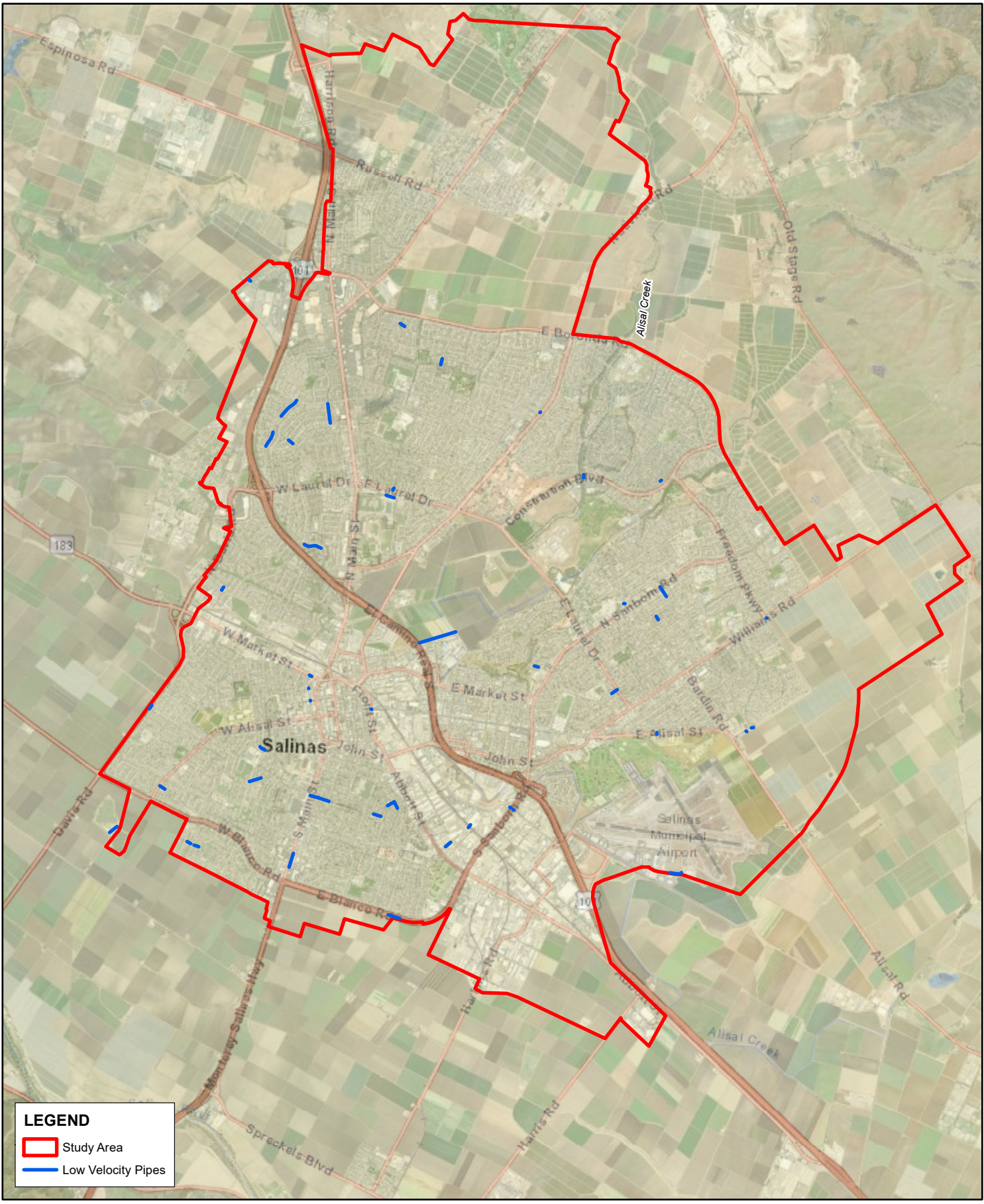
FIGURE D-3. PIPES WITH VELOCITY LESS THAN 2 FPS (5-YEAR 6-HOUR STORM, EXISTING CONDITIONS)
